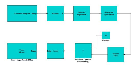
**Fig. S1. Block diagram of the Simulink MATLAB program for image processing.** After conversion of image stacks into a flattened image, a series of actions was applied to the image to acquire a binary edge detected map using MATLAB image processing toolbox. The detailed schematic view of used toolboxes and their order is depicted here for more information.
