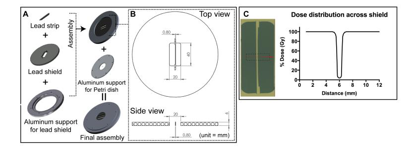
Figure S1. Parts and dimensions of lead shield assembly
