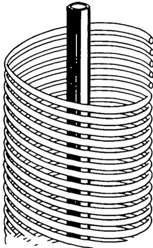
Fig. 1. Diagram of the sleeve showing 5 fibrils spiralling about a single remaining fibre.
