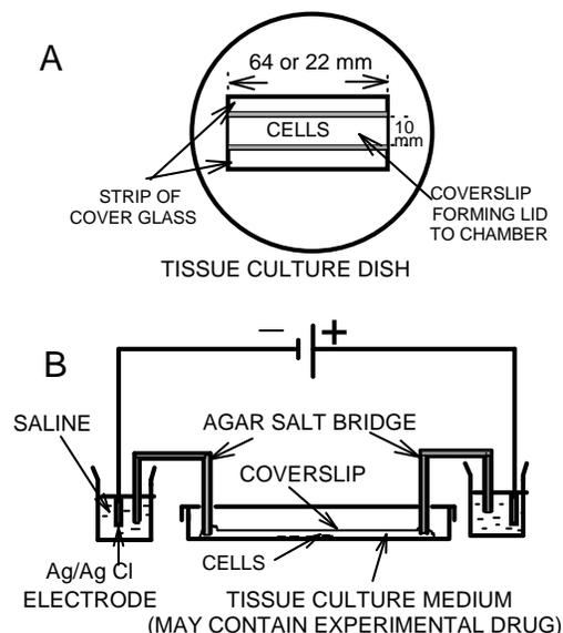
**Fig. 1.** Experimental design of culture chamber and field application. (A) Chamber constructed within a tissue culture plastic dish, viewed from above. (B) Side-on view includes dc power supply and Ag/AgCl electrodes isolated from the culture chamber using agar-gelled salt bridges.
