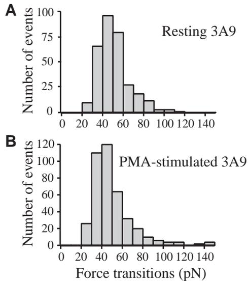
**Fig. 4.** Histograms of breakage forces of LFA-1-ICAM-1 bond(s) from the force-displacement traces of (A) resting and (B) PMA-stimulated 3A9 cells. The breakage forces were derived from the magnitude of the force transitions acquired in measurements obtained with a compression force of 200 pN, 5 seconds contact and a cantilever retraction speed of 2  $\mu\text{m}/\text{second}$ . The y-axis plots the number of force transitions detected.
