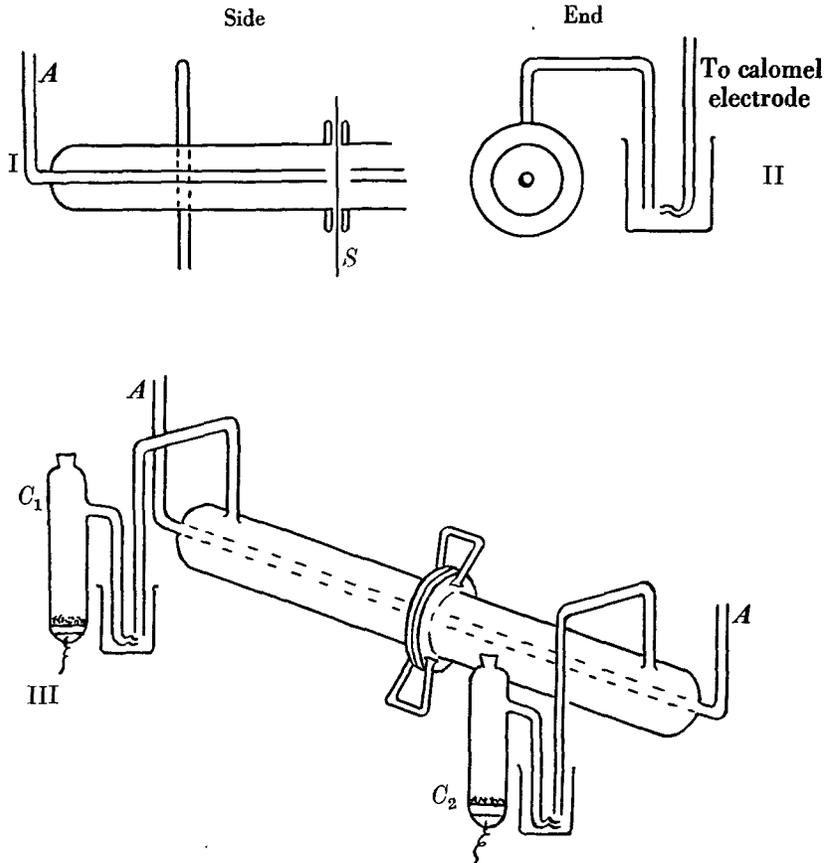
Fig. 1. Apparatus to measure potential of skin with calomel electrodes. I. Side view: *S*, skin; Solutions enter by *A*. II. End view showing siphon connection from cell to calomel electrode. III. Whole apparatus, skin and cell mounted with calomel electrodes  $C_1$ ,  $C_2$ .
