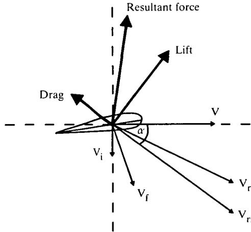
Fig. 2. Local velocity and force vectors at a wingchord in horizontal flight.  $V_{ri}$  is the resultant of the animal's flight speed,  $V$ , flapping velocity,  $V_f$ , and induced velocity  $V_i$ , while  $V_r$  is the resultant of  $V$  and  $V_f$ . The angle (the angle of incidence) between  $V_{ri}$  and the wingchord is  $\alpha$ .
