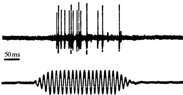
Fig. 1. Recording of activity from the statocyst crista nerve in response to a tone burst. The tone burst is at a frequency of 80 Hz and of 300 ms duration with 50 ms attack and decay times.
