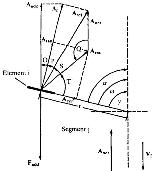
Fig. 4. The accelerative force ( $F_{add}$ ) of element i, located on segment j, is calculated. See text for explanation.
