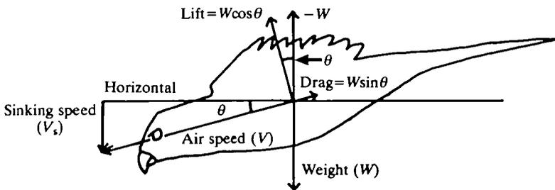
Fig. 1. Forces and velocities during equilibrium gliding. The glide path is inclined at glide angle  $\theta$  to the horizontal. Lift and drag are parallel and perpendicular, respectively, to the glide path. Air speed ( $V$ ) is parallel to the glide path, and sinking speed ( $V_s$ ) is vertical and downwards.
