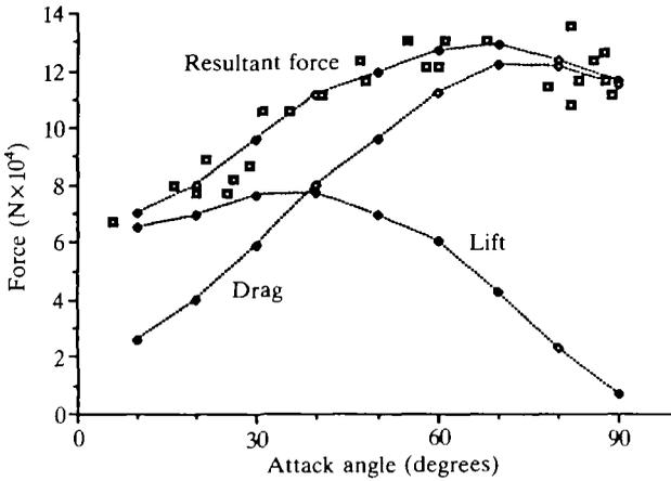
Fig. 2. Total (horizontal) aerodynamic force acting on a moderately large specimen of *Velella velella* (maximum sail length, 57 mm) at near-surface windspeeds of  $1.3 \text{ m s}^{-1}$ , measured as a function of the animal's orientation (attack angle of the sail). A line was fitted by connecting average points (small squares) calculated after rounding attack angles to the nearest  $10^\circ$ . Lift and drag components were calculated from direct measurements of force magnitude and direction.
