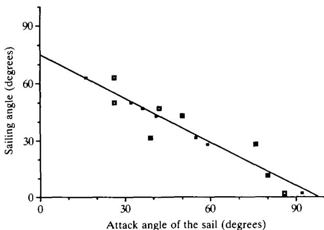
Fig. 5. Spontaneous orientation and sailing direction of eight freely sailing specimens of *Velella velella* measured in the wind tunnel. The line ( $y = -0.76x + 75.0$ ;  $r = 0.91$ ) was fitted to the data points (large squares) using least-squares regression. For comparison, attack angles producing a resultant force in the direction of motion (taken from static test results) are also given for each animal (small squares).
