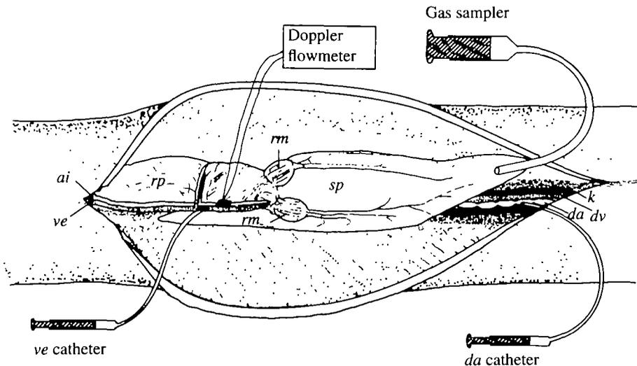
Fig. 1. Schematic drawing of the eel swimbladder preparation showing the location of the various catheters. *ai*, arterial influx; *da*, dorsal artery; *dv*, dorsal vein; *k*, kidney; *rm*, rete mirabile; *rp*, resorbing part of the swimbladder; *sp*, secretory part of the swimbladder; *ve*, venous efflux.
