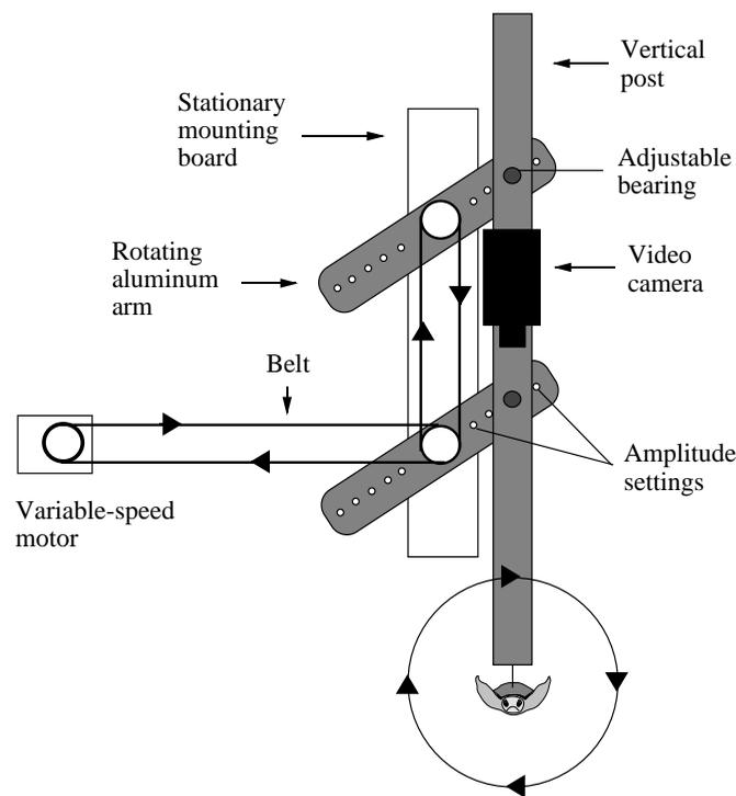
Fig. 3. Diagram of the wave motion simulator used to simulate the orbital movements that occur beneath small oceanic waves (Lohmann *et al.* 1995). A small, variable-speed motor turned a belt, which in turn drove two identical acrylic arms coupled by a second belt. As the arms rotated, they remained parallel to each other and moved a vertical post (with a hatchling attached to the bottom) through a series of circular movements.
