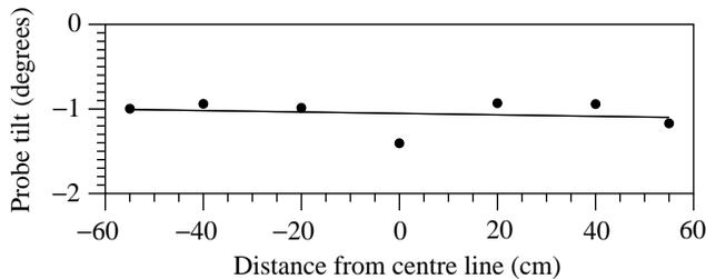
Fig. 7. Tilt angle, as measured by the X-wire probe (see Fig. 4B), across the centre line of plane 2 (see Fig. 5), with the tunnel horizontal ( $r=-0.192$ ). Equivalent air speed was  $10 \text{ m s}^{-1}$ .
