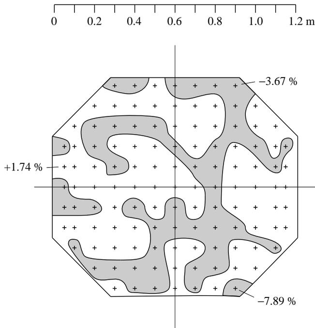
Fig. 3. Survey of equivalent wind speed in the wind tunnel, using a pitot-static probe placed at 119 points (crosses) in plane 4 (see Fig. 5). The wind speed was below the mean ( $21.28 \text{ m s}^{-1}$ ) at all points in the shaded area and above the mean at the points in the white area. The positions of three points where the wind speed deviated from the mean by anomalously large amounts are indicated. Speeds at the other 116 points deviated by less than 1.3% from the mean.
