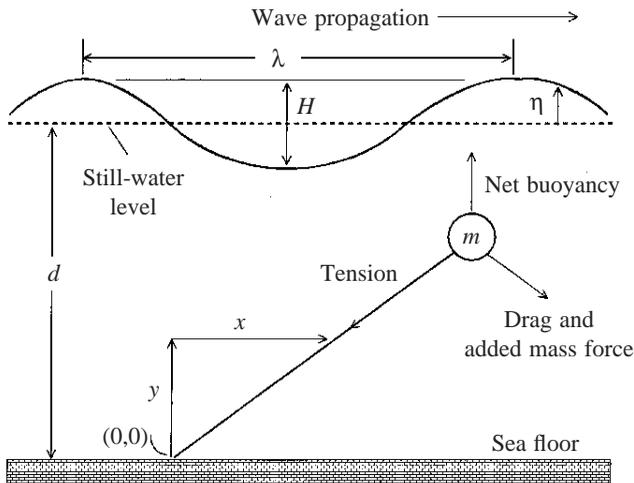
Fig. 2. A schematic representation of the numerical model of kelp dynamics. For further details, see the text.  $d$ , water column depth;  $H$ , wave height;  $\eta$ , vertical deviation from still-water level;  $m$ , plant mass;  $x$ ,  $y$ , horizontal and vertical coordinate axes, respectively;  $\lambda$ , wavelength.
