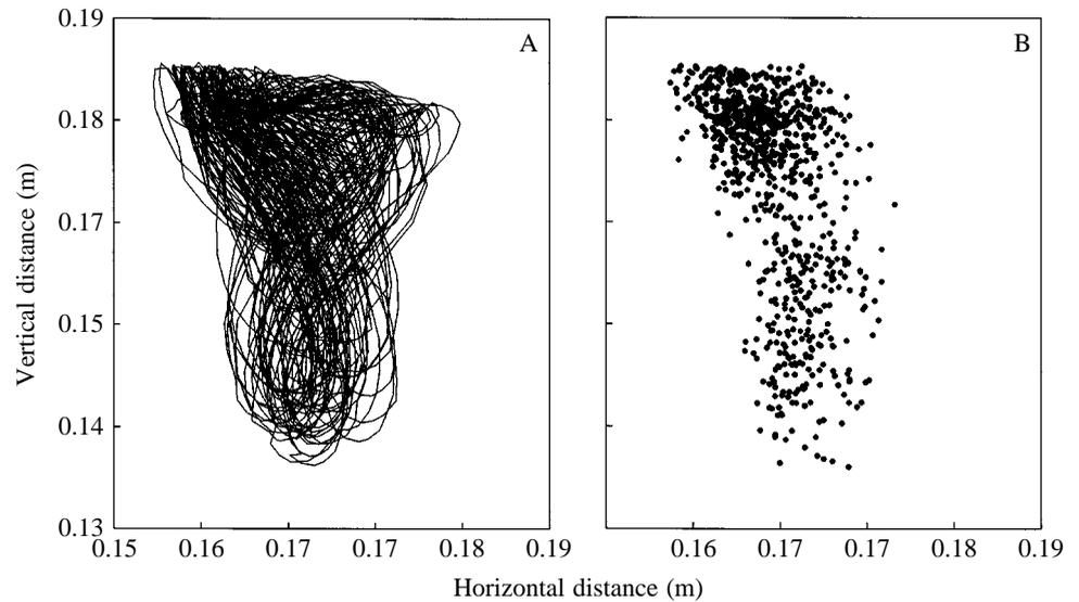
The largest Lyapunov exponent for the measured motion of the corn-oil-filled ball is positive:  $0.317 \pm 0.055$  (95% confidence limits) for  $x$ -directed motion and  $0.158 \pm 0.052$  for  $y$ -directed motion, indicative of chaos. The largest Lyapunov number calculated for data from our numerical predictions is also positive:  $0.304 \pm 0.038$  (95% confidence limits) for  $x$ -
