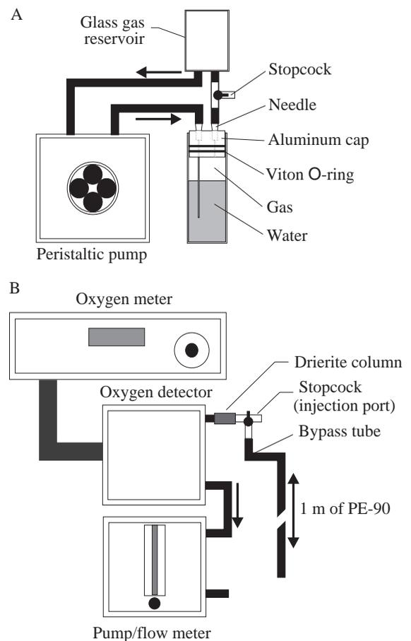
Fig. 1. A schematic representation of the respirometer (A) and oxygen analyzer with modified bypass tube (B) used to measure  $\dot{M}_{O_2}$  in aquatic *Xenopus laevis* (for a detailed description, refer to Materials and methods).
