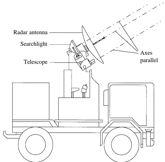
Fig. 2. The tracking radar 'Superfledermaus' with its telescope and an additional strong searchlight mounted parallel to the axis of the parabolic radar antenna. An infrared camera could be mounted instead of the searchlight.
