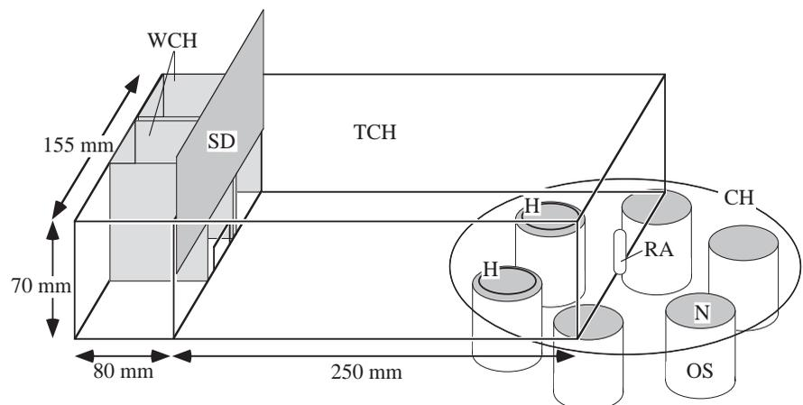
Fig. 1. A diagram of the experimental apparatus. WCH, waiting chambers; TCH, training chamber; CH, container holder; RA, rotating axle; OS, odour source; N, gauze net; SD, sliding door; H, holes connecting the chamber with two of the six odour sources.
