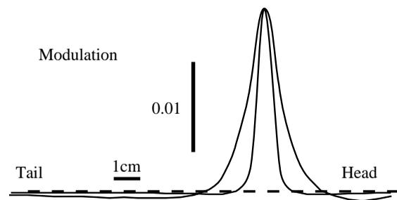
Fig. 8. Distance is coded by the spatial peak-to-peak (PP) amplitude profile but not by the PP amplitude at the projection point. The graph compares two PP modulation profiles generated by two elementary objects of different resistance when placed at the appropriate distance to produce the same local electric organ discharge (LEOD) at the projection point. Note the difference in relative slope.
