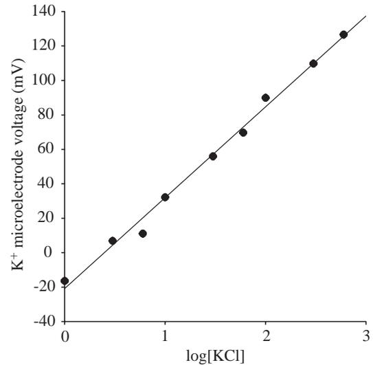
Fig. 2. Calibration curve for  $K^+$  microelectrodes in KCl solutions of 1–600  $\text{mmol l}^{-1}$ . Data points are mean responses  $\pm$  S.E.M. of four different electrodes; standard errors are smaller than the symbol used. The solid line (slope 52.7 mV per decade) is the linear regression ( $r^2=0.992$ ,  $P=0.0002$ ).
