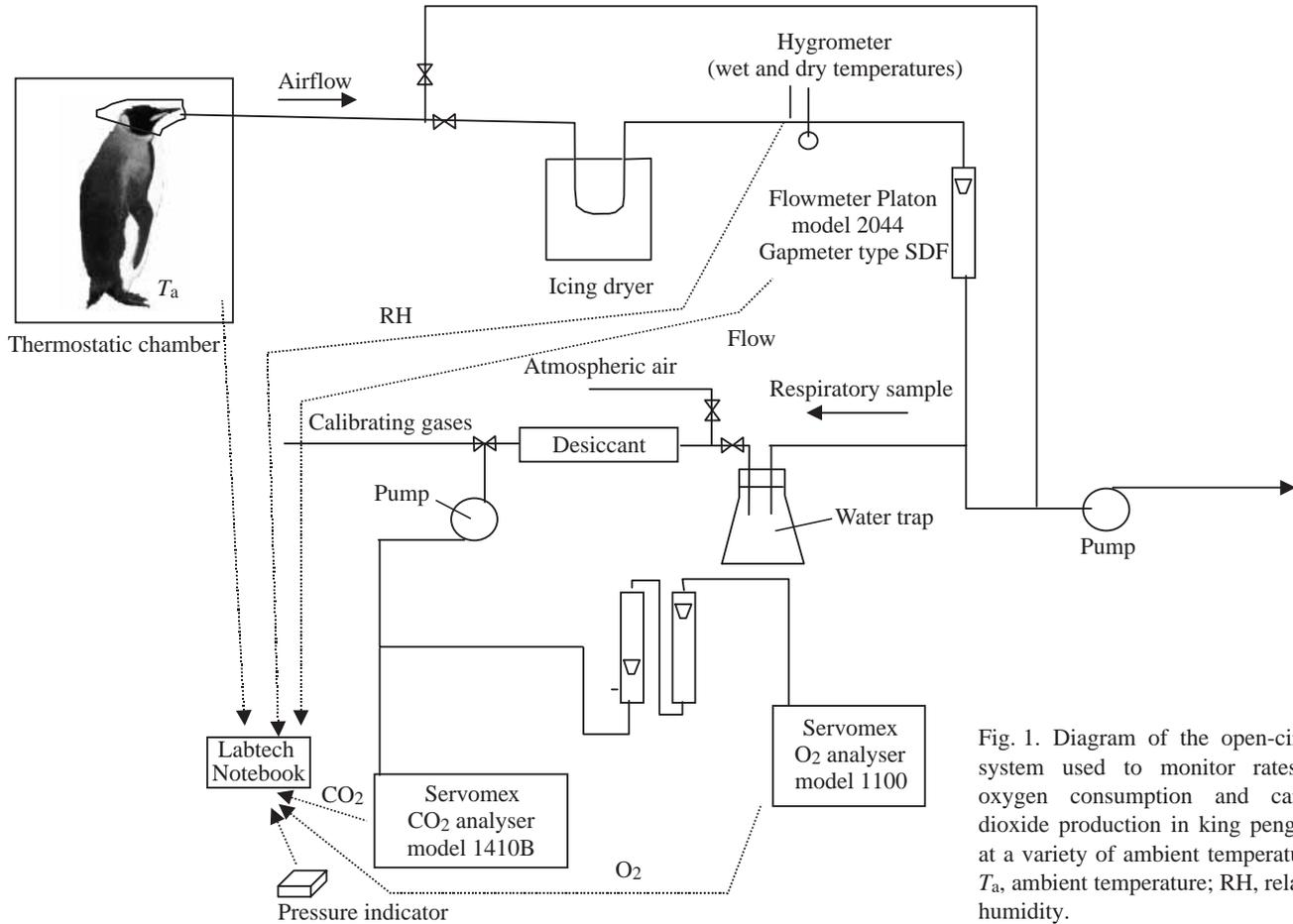
Fig. 1. Diagram of the open-circuit system used to monitor rates of oxygen consumption and carbon dioxide production in king penguins at a variety of ambient temperatures.  $T_a$ , ambient temperature; RH, relative humidity.
