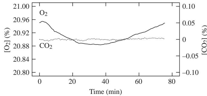
Fig. 6. Typical example of changes in baseline O<sub>2</sub> and CO<sub>2</sub> concentration occurring while heliox was circulated through an empty metabolic chamber. Five other trials were conducted, and all yielded similar results.
