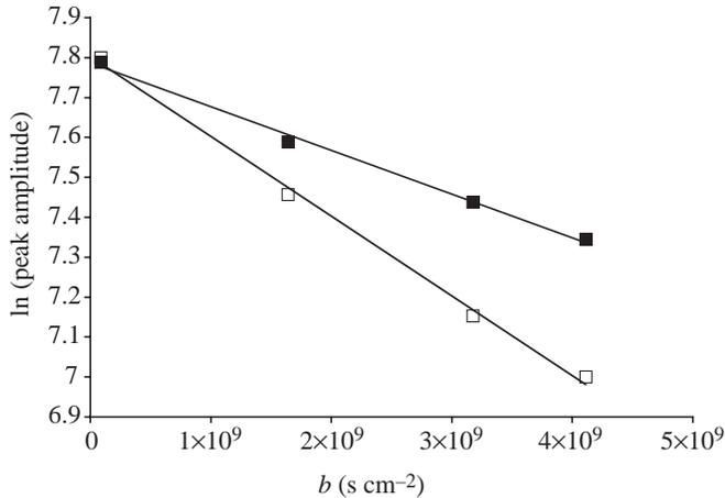
Fig. 3. Typical attenuation plot of the NMR peak amplitude as a function of the diffusion-weighting factor  $b$  in the axial (open squares) and radial (filled squares) directions in *P. argus* muscle. This example is from a measurement of arginine phosphate diffusion at a diffusion time of 150 ms. A steeper attenuation slope is indicative of a higher  $D$ , as seen for axial diffusion.
