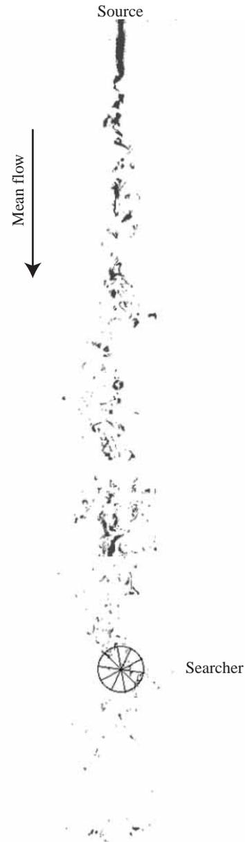
Fig. 1. Illustration of a simulated searcher in the chemical plume. The searcher's ten sensors are located at the ends of the 'spokes'. The dark patches are areas where the chemical stimulus is above threshold. The image is to scale, with the plume extending approximately 150 cm downstream of the source and the diameter of the searcher equal to 10 cm.
