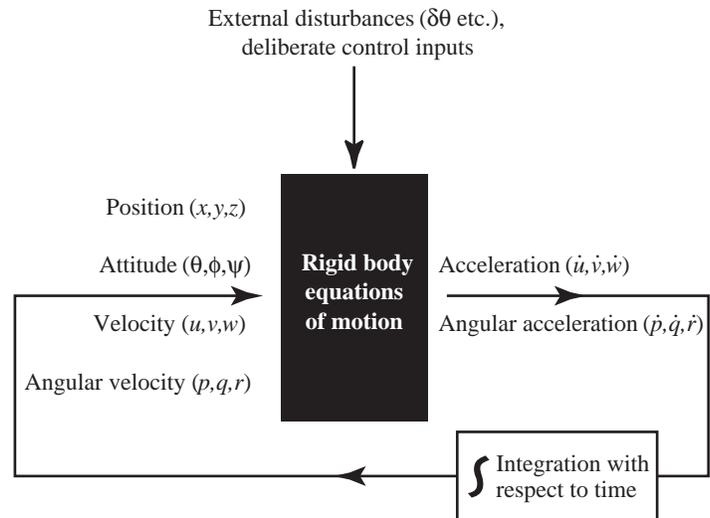
Fig. 1. Black box representation of the rigid body equations of motion underpinning the quantitative framework of this analysis. The integral sign represents a bank of single integrators.
