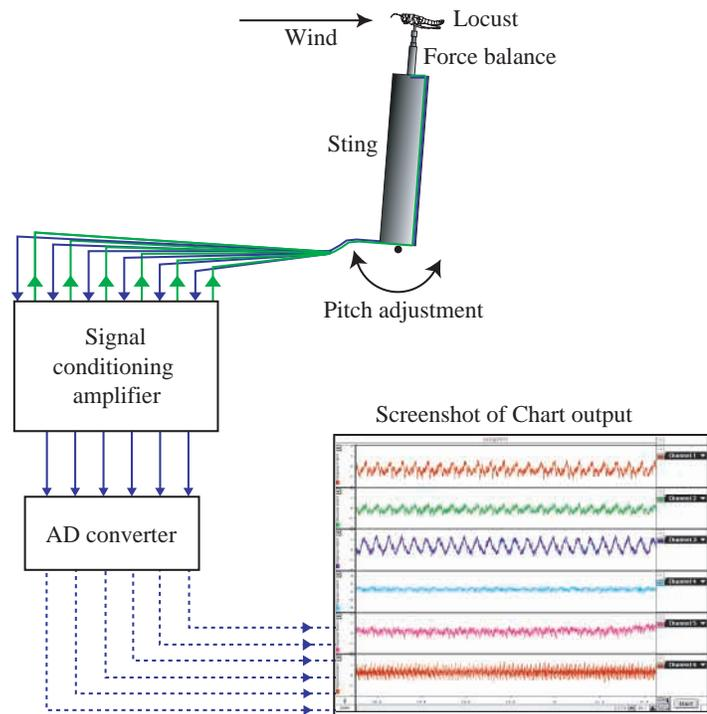
Fig. 3. Schematic representation of the experimental setup. AD, analogue-to-digital.
