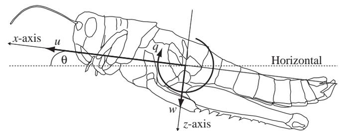
Fig. 2. Definition of the state variables  $u$ ,  $w$ ,  $q$  and  $\theta$ . Each of the variables is signed positive in the direction shown. The body axes are centred upon the centre of mass and are aligned so that the  $x$ -axis points in the direction of flight at equilibrium. The locust is shown during a nose-up perturbation:  $q$  is zero at equilibrium, and  $w$  and  $\theta$  are defined so as to be zero at equilibrium.
