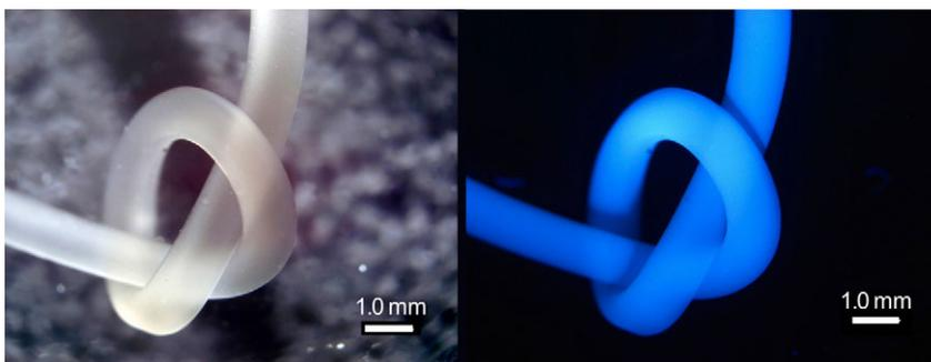
Fig. 2. Bio-synthesised resilin moulded into a flexible rod by drawing pro-resilin into a glass tube, followed by photochemical cross-linking of the precursor. Left, the rod illuminated by white light. Right, the same rod illuminated by U.V. light at 315 nm showing its fluorescence at 409 nm. Figure reproduced from Elvin et al. (Elvin et al., 2005) with permission: photograph by Dr David Merritt, UQ, Brisbane, Australia.
