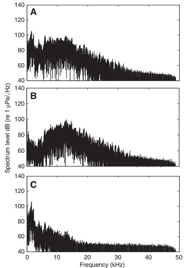
Fig. 1. Power spectra comparison of the 0.2–20 kHz (A), 6–20 kHz (B) and 0.2–2 kHz (C) broadband test signals played at the 3000 ms duration (sample rate of 97,656 Hz).
