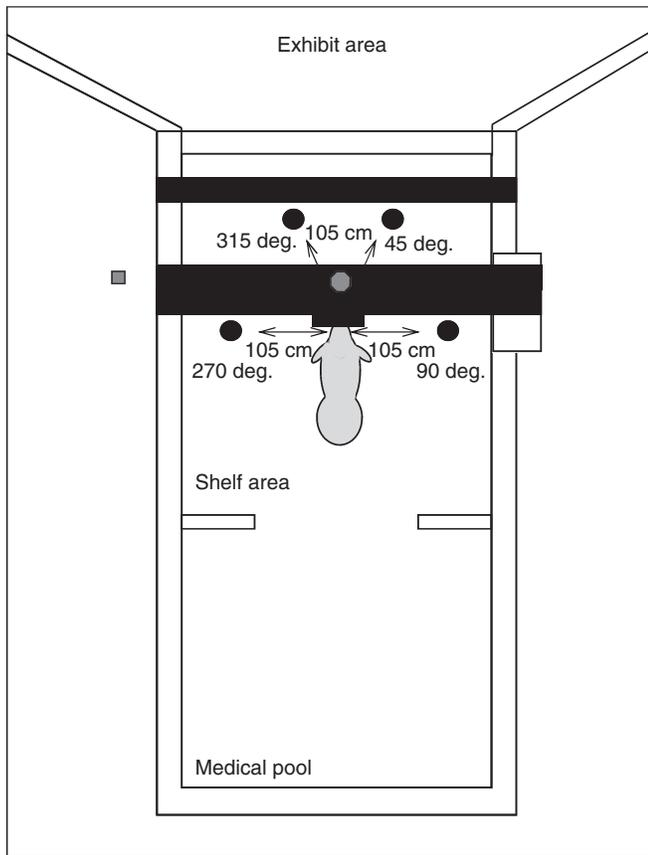
Fig.2. Testing configuration with four test speakers located 105cm from the center of the stationing bar and 75cm below the surface. The test speakers are represented as the black circles. The gray octagon represents the 'test trainer's' position and the gray square represents the 'data recorder's' position.
