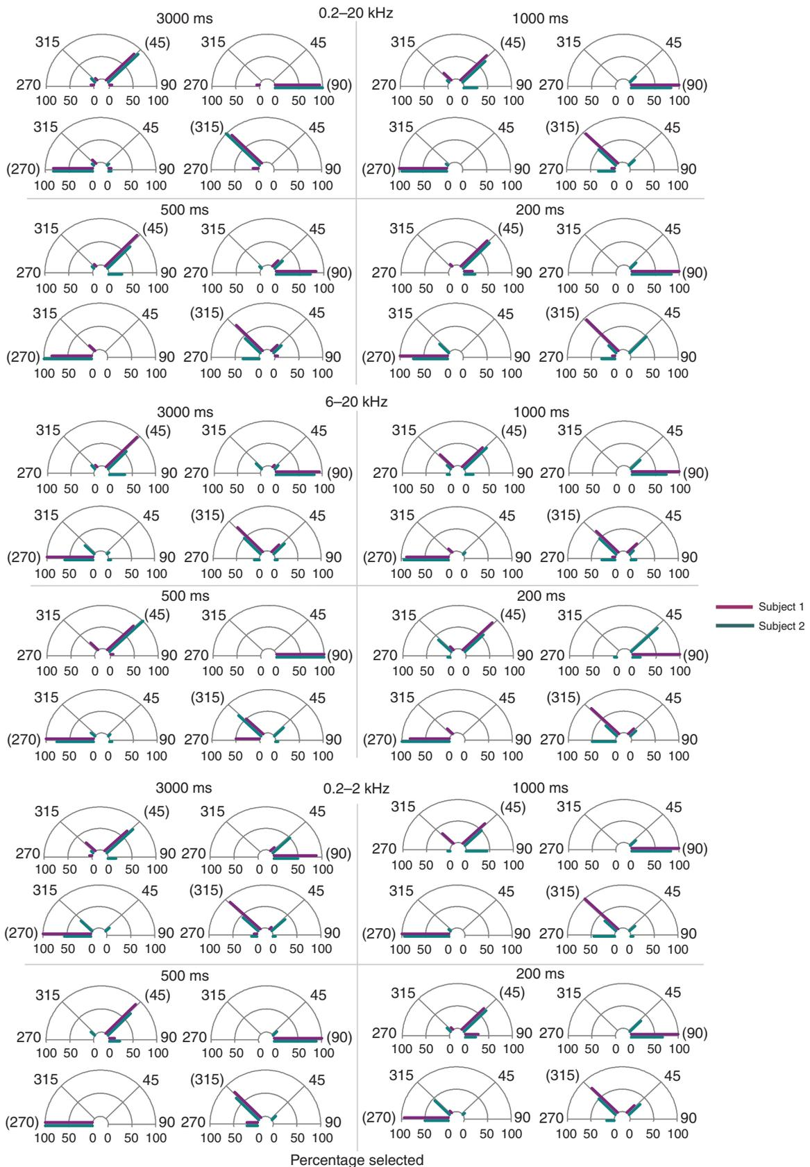
Fig. 5. Percentage correct and distribution of errors by duration within the 0.2–20 kHz, 6–20 kHz and 0.2–2 kHz broadband conditions. Correct speaker location is notated by parentheses. Subject 1's results are presented above the grid lines and Subject 2's are presented below.
