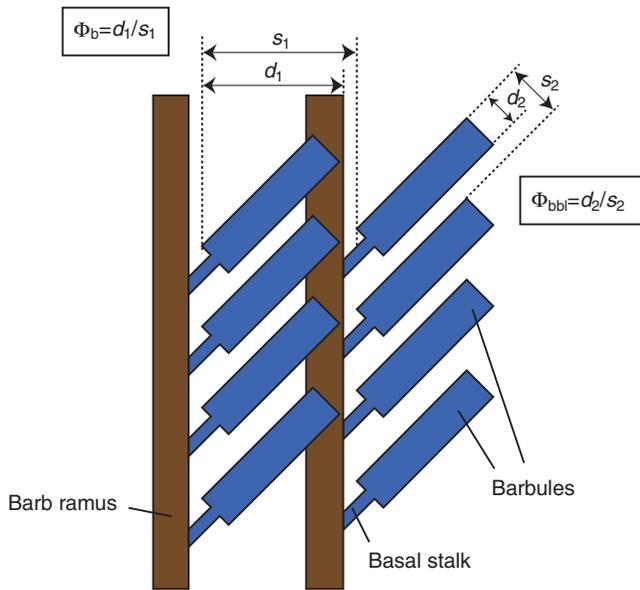
Fig. 2. Schematic drawing of the dorsal surface of an iridescent mallard feather showing iridescent barbules (blue) and barb ramus (brown). The surface fraction of keratin ( $\phi$ ) is calculated as width ( $d$ ) divided by spacing ( $s$ ) for both barbs and barbules. Note that the surface of the basal stalk is lower (further into the paper) than the surface of the distal region (blue rectangle) of the iridescent barbules. For simplicity, only exposed (distal) barbules are shown.
