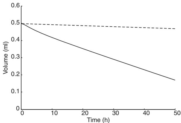
Fig. 6. Model of changes in volume of a diving bell, assuming an initial volume of 0.5 ml at 100 mm depth. Volume decreases of an empty bell (dashed line) and with a 50 mg spider (solid line) are shown. The model incorporates empirical data on the relationships between volume and conductance and the metabolic rate of the resting spider.
