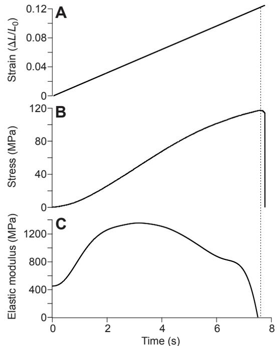
Fig. 2. Sample strain (A) and stress (B) measurements for a turkey FPPD3 tendon. Data are for a controlled isovelocity lengthening at  $1 \text{ mm s}^{-1}$ . Continuous elastic modulus (EM; C) was measured as the derivative of stress over strain. Maximum EM was determined by taking the peak of the continuous EM curve (C). Breaking stress and strain were taken at the point of maximum stress, as indicated by the dotted line.
