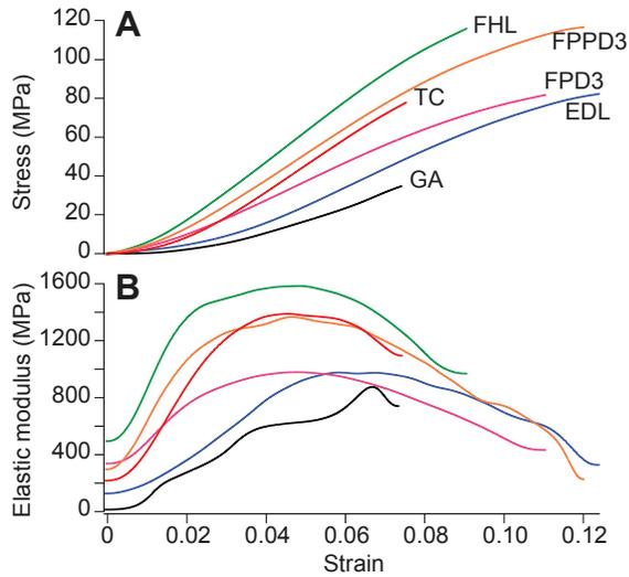
Fig. 3. Stress–strain relationships (A) and continuous elastic moduli (B) for six different tendons in a single turkey hindlimb specimen. Colors in B are as labelled in (A).
