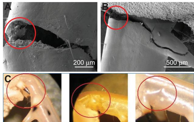
Fig. 3. Selection of failure modes of locust tibiae. (A,B) Scanning electron microscopy images showing failure by cracking on the tensile side of tibiae after fatigue testing. The circles indicate the area of crack initiation. (C) Evidence of failure by buckling on the compressive side of tibia samples.
