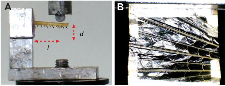
Fig. 1. Experimental setup for cyclic loading of locust legs and wings. (A) The proximal end of the tibia is fixed, whilst the actuator presses down a deflection amplitude  $d$  at a distance  $l$  from the clamping. (B) The aluminium foil frame with the wing section is mounted between two standard tensile clamps. Before the test, the connecting parts of the frame are cut. Both tibia and wing samples were fully submerged in water during the tests (container not shown).
