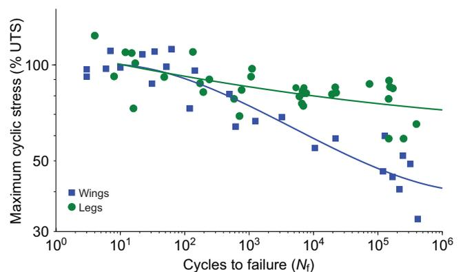
Fig. 2. Fatigue test results, showing the number of cycles to failure as a function of the maximum stress in the cycle, expressed as a percentage of the ultimate tensile strength (UTS). The lines present the best fit for a typical sigmoidal fatigue curve model (for details, see Results).
