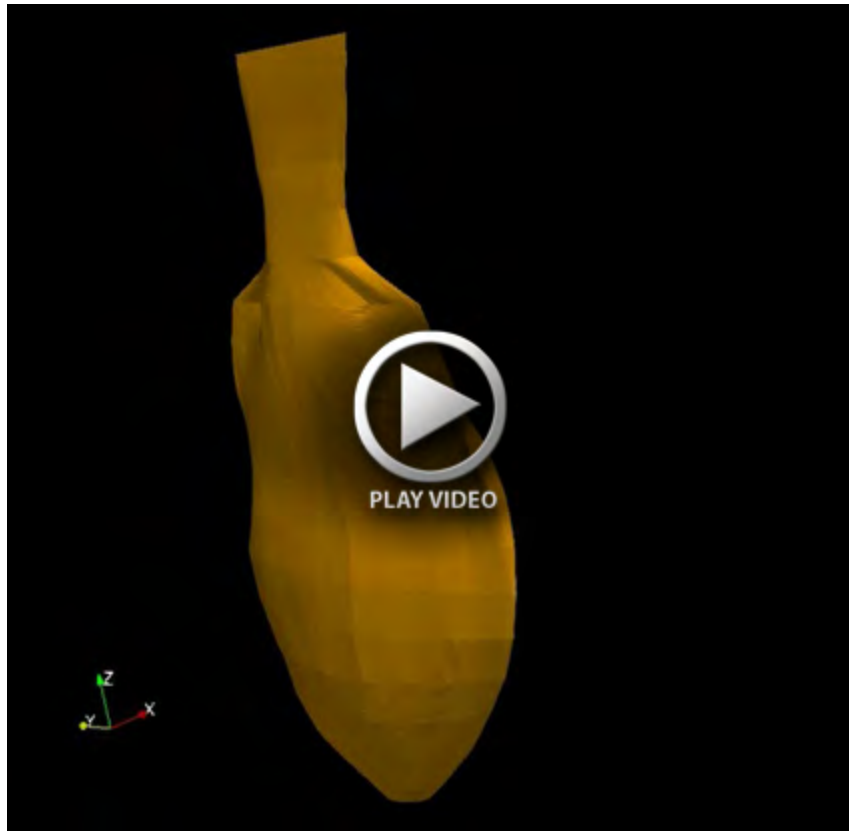
Movie 1. Sunfish with no anal/dorsal fins. The 3D wake structure visualized using iso-surfaces of q-criteria for the sunfish with no anal/dorsal fins ( Re=4000 simulation).
