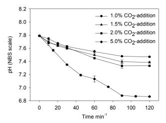
**Fig. S3.** Stability of the live-cell CO<sub>2</sub> incubator after different levels of CO<sub>2</sub> addition. pH (NBS scale) was calculated using a spectro-photometer following the m-cresol dye method, stipulated in SOP 6B (Dickson et al., 2007).
