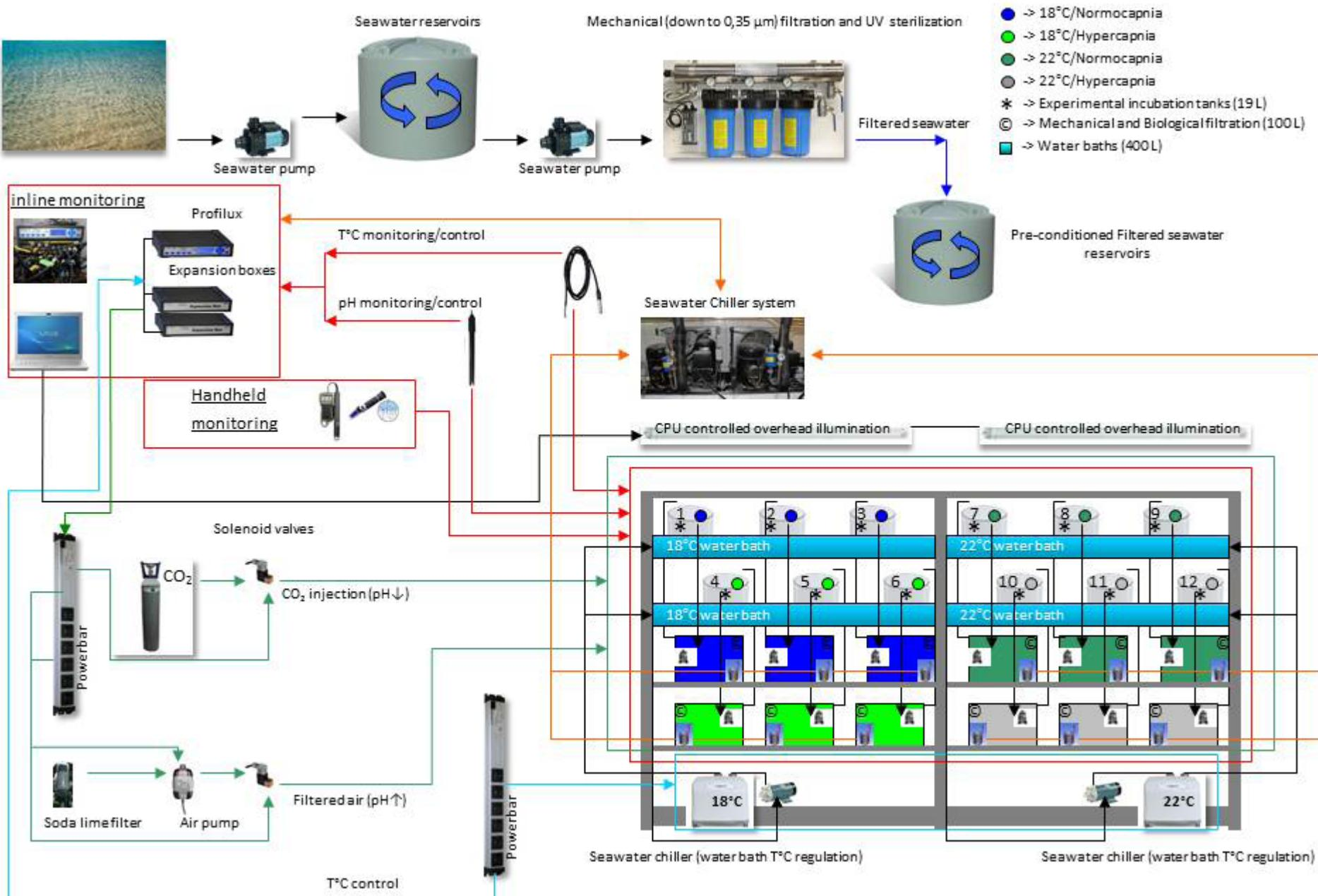
**Fig. S1.** Schematics of the experimental setup used to perform experimental exposure of *Solea senegalensis* larvae to ocean warming and acidification.
