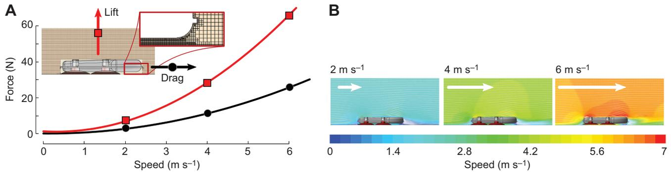
**Fig. 4. Lift and drag forces on a DTAG2 increase with speed.** (A) Lift (red) and drag (black) forces (N) on a DTAG2, and (B) flow visualization at uniform velocity profiles of 2, 4 and 6 m s<sup>-1</sup> from computational fluid dynamics (CFD) simulations using STAR-CCM+ (version 9.04) over 9.6 m cells, with extra mesh refinement in the region located under the tag (A). See main text for further CFD details.
