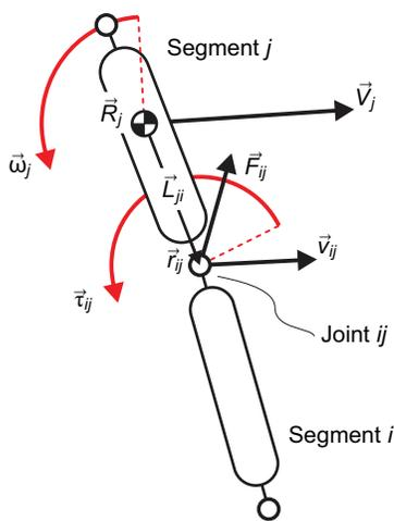
**Fig. A2. Example of a linked chain of segments.** Vectors are joint force  $\vec{F}_{ij}$ , joint torque  $\vec{\tau}_{ij}$ , CoM position  $\vec{R}_j$  of segment  $j$ , position  $\vec{r}_{ij}$  of joint  $ij$ , vector  $\vec{L}_{ji}$  from  $\vec{R}_j$  to  $\vec{r}_{ij}$ , CoM velocity  $\vec{V}_j$  of segment  $j$ , velocity  $\vec{v}_{ij}$  of joint  $ij$ , and angular velocity  $\vec{\omega}_j$  of segment  $j$  around its CoM.
