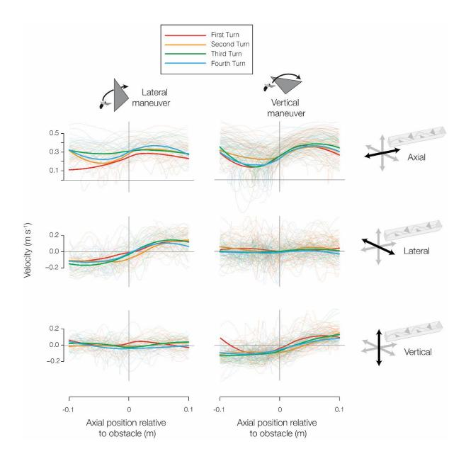
Fig. S5. Axial (top), lateral (middle), and vertical (bottom) velocity *vs.* position relative to the obstacle, with obstacles separated by the order in which they were encountered. Red, orange, green, and blue lines represent maneuvers performed to avoid the first, second, third, and fourth obstacles encountered during a given trial. Thickened lines show average velocity *vs.* position (from local regression smoothing) for each turn, and thin transparent lines show individual traces.
