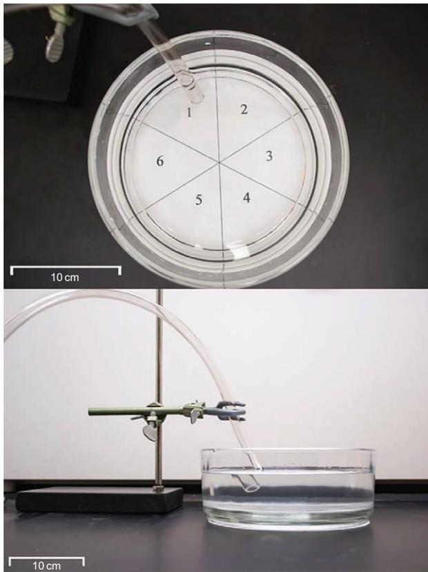
**Fig. 3. Experimental set up for exposing different water flow rates to *C. pettiti* and *H. morosa* larvae.** The airflow tube was fixed to an airflow detector/regulator attached to a laboratory source of filtered compressed air. Photo credit: B. Nelson and L. Main.
