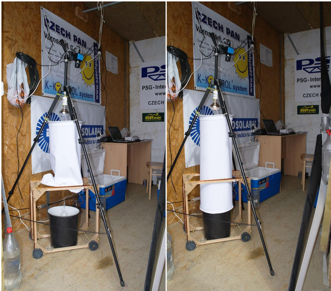
Fig. S2. Laboratory in polar station and testing device. Set-up with white cloth shielding lifted for manipulation with animals (left). White tunnel pulled down for testing (right). Note position of white testing dish (shown with no water) and releasing funnel in the middle which can be lifted from above by a string. Illumination and camera from above, wooden Helmholtz coil on the floor, blue tank as animal store, table with PC and power supply behind also apparent.
