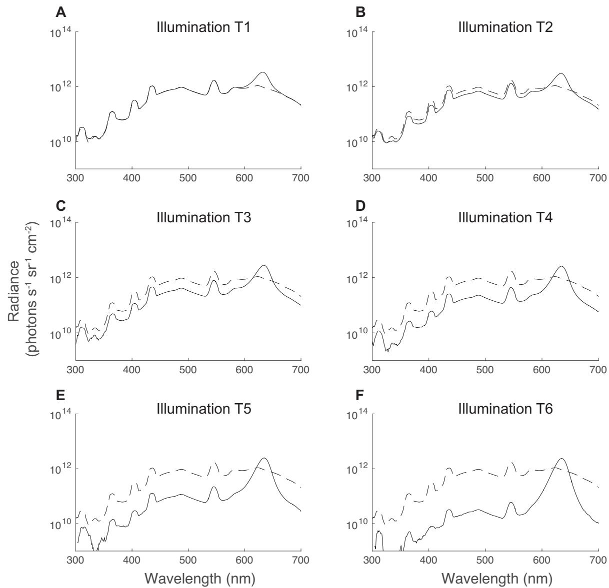
**Fig. S1. Spectral radiance of all illuminations.** The radiance of the illuminations as measured from a white standard placed on the floor of the experimental arena. The white control illumination is plotted as a dashed line in all panels.
