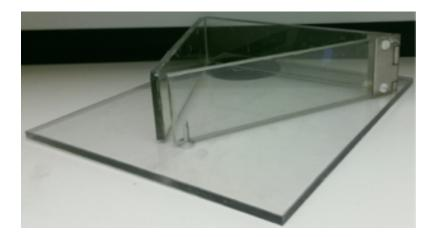
Figure S1. Custom-built enclosure with adjustable slit-shaped aperture. The enclosure was placed into a large cooler filled with artificial seawater, and hagfishes were placed, one at a time, into the enclosure and observed from above as they attempted to escape through the slit. A glass lid (not shown) allowed filming from above. The enclosure had dimensions of 0.203 m x 0.0508 m x 0.176 m for a total of 1.17 m<sup>3</sup>.
