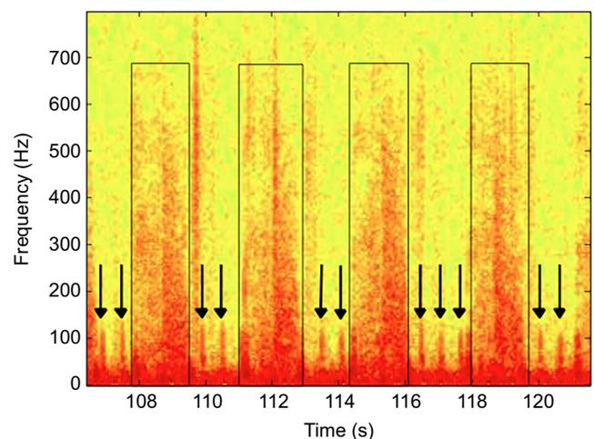
**Fig. 1. Spectrogram of recorded sound.** Data were obtained from a southern elephant seal (seal 1) during a surface interval, and show four respiratory cycles (rectangles in the 0–700 Hz range) with cardiac occurrences between breaths (black arrows in the 0–150 Hz range).
