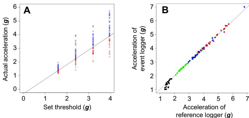
**Fig. 1. Calibration of the detection accelerometer.**
