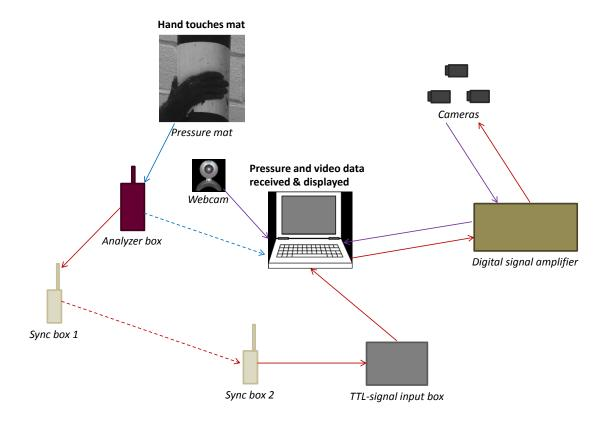
**Fig. S1**: Illustration of the technical set-up. Grasping of the pressure mat results in both the generation of pressure data and the initiation of the synchronisation signal which triggers the high-speed cameras to record. Blue arrows – route for pressure data transfer. Maroon arrows – route for synchronisation signal transfer. Purple arrows – route for visual data transfer. Solid arrows reflect a direct, wired connection whilst dotted arrows are for Bluetooth connections.
