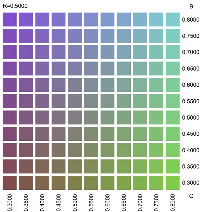
**Fig. 2. Colour matrix with specific RGB values created using the `GetRGBcombinations.m` code.** Colours were printed with a laserjet printer and the spectral reflectance of each colour combination was measured with a spectrophotometer. All the colours in this matrix have an R value of 0.5. The G and B values are shown on the x-axis and y-axis, respectively. We made additional sample colours with other R values ranging from 0 to 1 to make the gamut of experimental colours.
