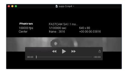
Movie 2. Typical high-speed video in recording the dynamic in-out bending of shell sample from its lateral view. The shell sample was shown in the middle of the field of view. The loading part of the impact tester translated from left to right in the video. Its velocity values before bending and after sample fracture were calculated by the movement of the white marker on its top surface.
