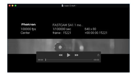
Movie 1. Typical high-speed video in recording the dynamic out-in bending of shell sample from its lateral view. The shell sample was shown in the middle of the field of view. The loading part of the impact tester translated from left to right in the video. Its velocity values before bending and after sample fracture were calculated by the movement of the white marker on its top surface.
