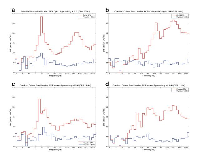
**Figure S1**. One-third-octave band levels for radiated noise from RHIB *Ziphid* during close approaches (~100m) to recording buoys at controlled speeds of 5 kt (panel a) and 10 kt (b) and from RHIB *Physalus* during close approaches (~100m) to recording buoys at controlled speeds of 5 kt (c) and 10 kt (d)
