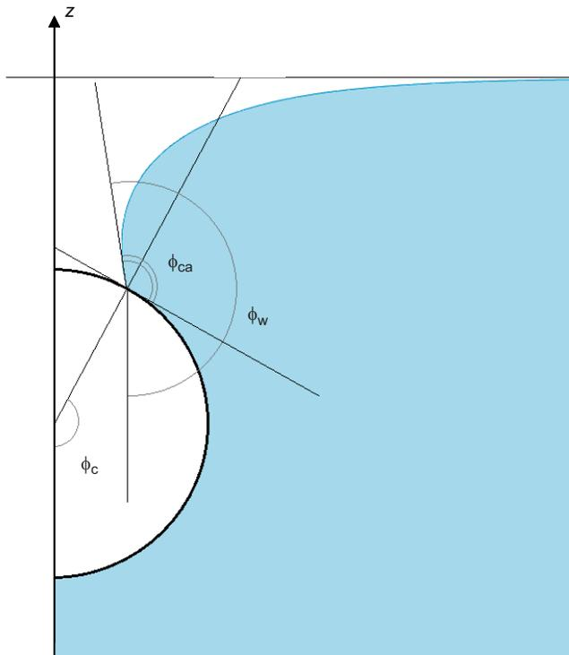
**Fig. 3. Cylindrical body (just one half is shown) submerged in water (shown in blue).** The undisturbed water level is at  $z=0$ ,  $\phi_{ca}$  is the water contact angle,  $\phi_c$  is the angle between the  $z$ -axis and a line going through the center of cylinder and the point of the water meniscus contact on the cylinder, and  $\phi_w$  is the angle between the water meniscus surface and a vertical.
