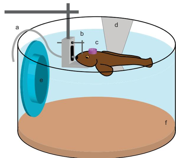
**Fig. 2. Schematic representation of experimental physiology tank.** For each physiology experiment, a fish was affixed and suspended 4 cm below the water's surface with the otic capsule 10 cm perpendicular from the face of the underwater speaker (e). Labels are as follows: a, respiration tube; b, head holder; c, hydrophobic water dam; d, Parafilm sling; f, sediment. Physiology tank dimensions: 40 cm diameter, 20 cm water depth.
