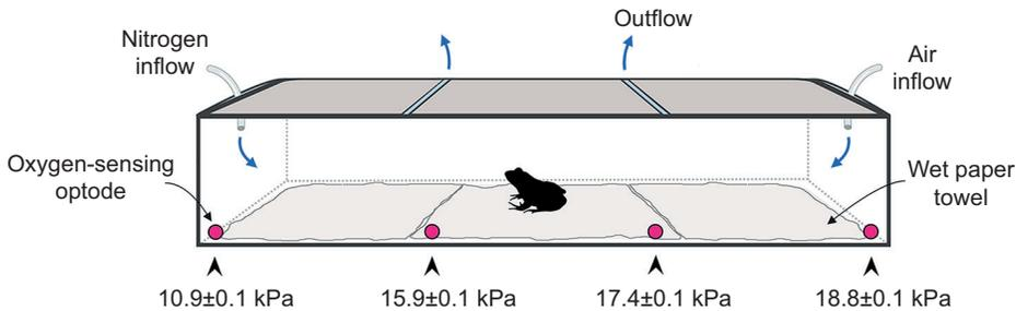
**Fig. 1. Schematic representation of a custom-built experimental choice chamber.** The partial pressure of  $O_2$  ( $P_{O_2}$ ) range within the low  $O_2$  zone (left), medium  $O_2$  zone (centre) and high  $O_2$  zone (right) was determined using  $O_2$ -sensing optodes and a Presens Optical Oxygen Sensor. The choice chambers used for *Cyclorana alboguttata* were 750×240×120 mm and made from clear acrylic.
